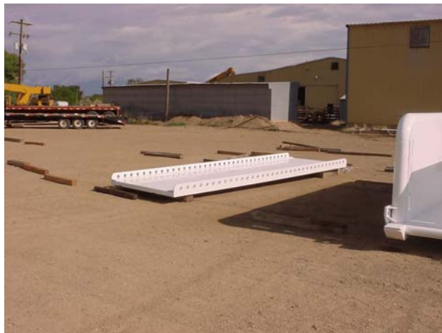
Electrical reel tray to be hauled with shield hauler .
