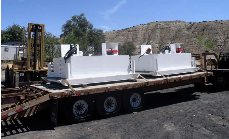
Fuel skid for refueling underground. Can be supplied with air or hand pump.
