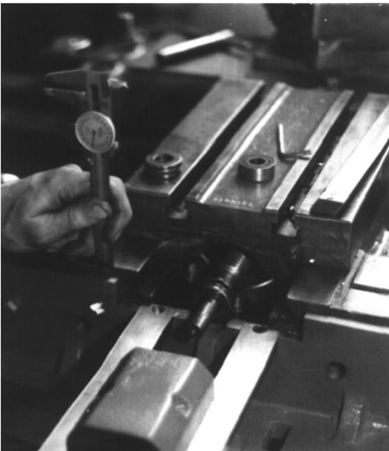
Next, bolt the taper attachment to the rear of the saddle in such a position that the cross slide screw would, if it were longer, pass directly through the center of the screw anchor block. (This is the part which the machinist holds in his left hand in Fig. C). Drill the mounting holes a little oversize so that the taper attachment can be leveled accurately with the saddle using a pair of vernier calipers or a depth micrometer as shown (Fig. A) is Fig.
