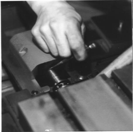
After locating the point for the hole to be drilled in the screw anchor block, remove it from the taper attachment in the manner shown in Fig. C. Drill the hole to the diameter of the end of the telescoping screw, or to some other suitable size that you determine. You may want to make it slightly oversize if you have made any errors in finding the point to be drilled. You may also wish to counter bore the hole on both ends to protect the thrust bearings, but this is not a must.
