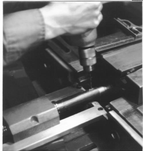
saddle is moved lengthwise. (The clamp must be fastened to the ways and the bottom slide while this is being done, just as if you were cutting a taper.) When you have found zero degrees of taper, make a mark on both ends of the bottom slide to correspond with the zero marks on the top slide.
