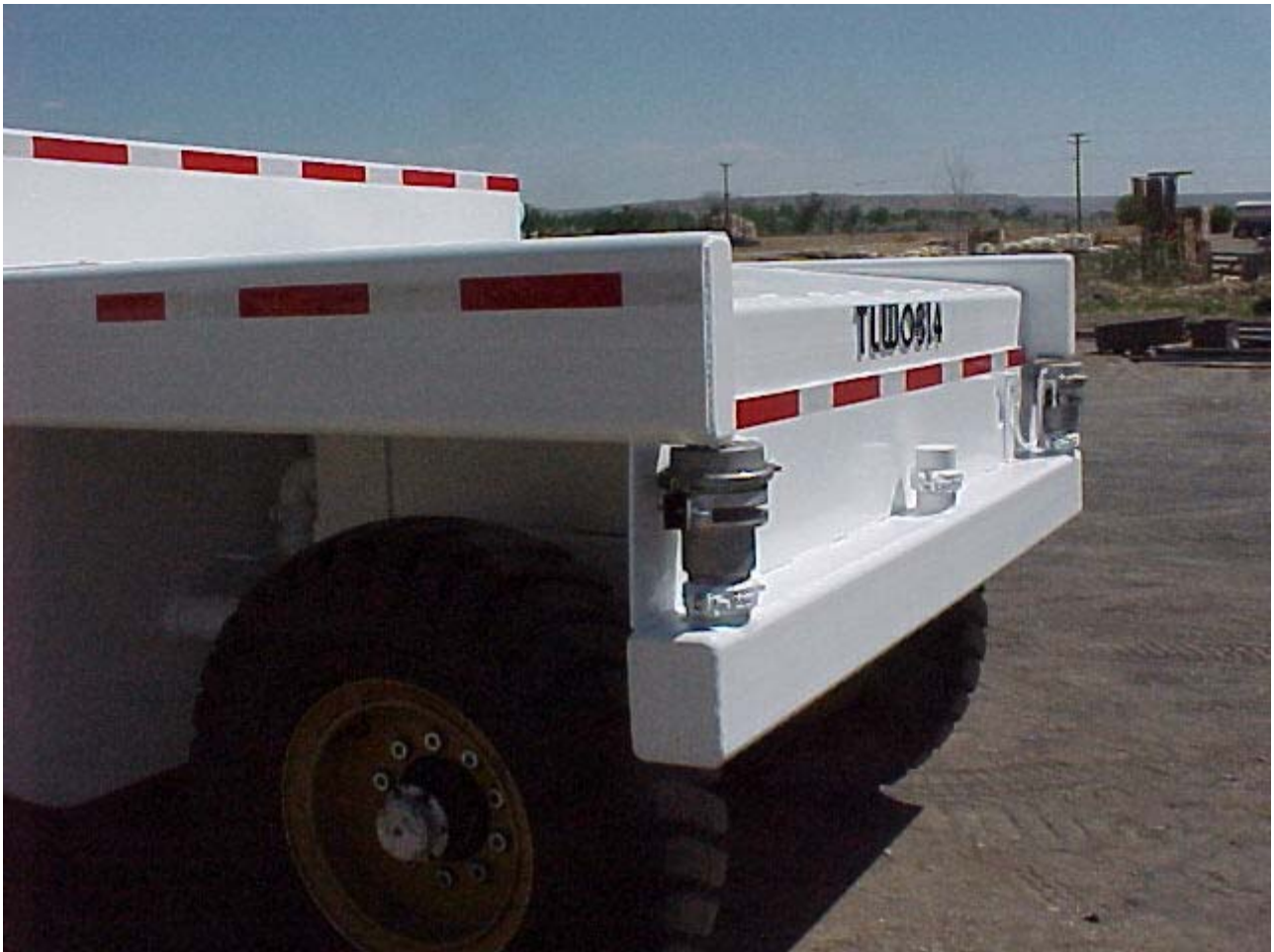
Rear of water wagon showing spray heads
