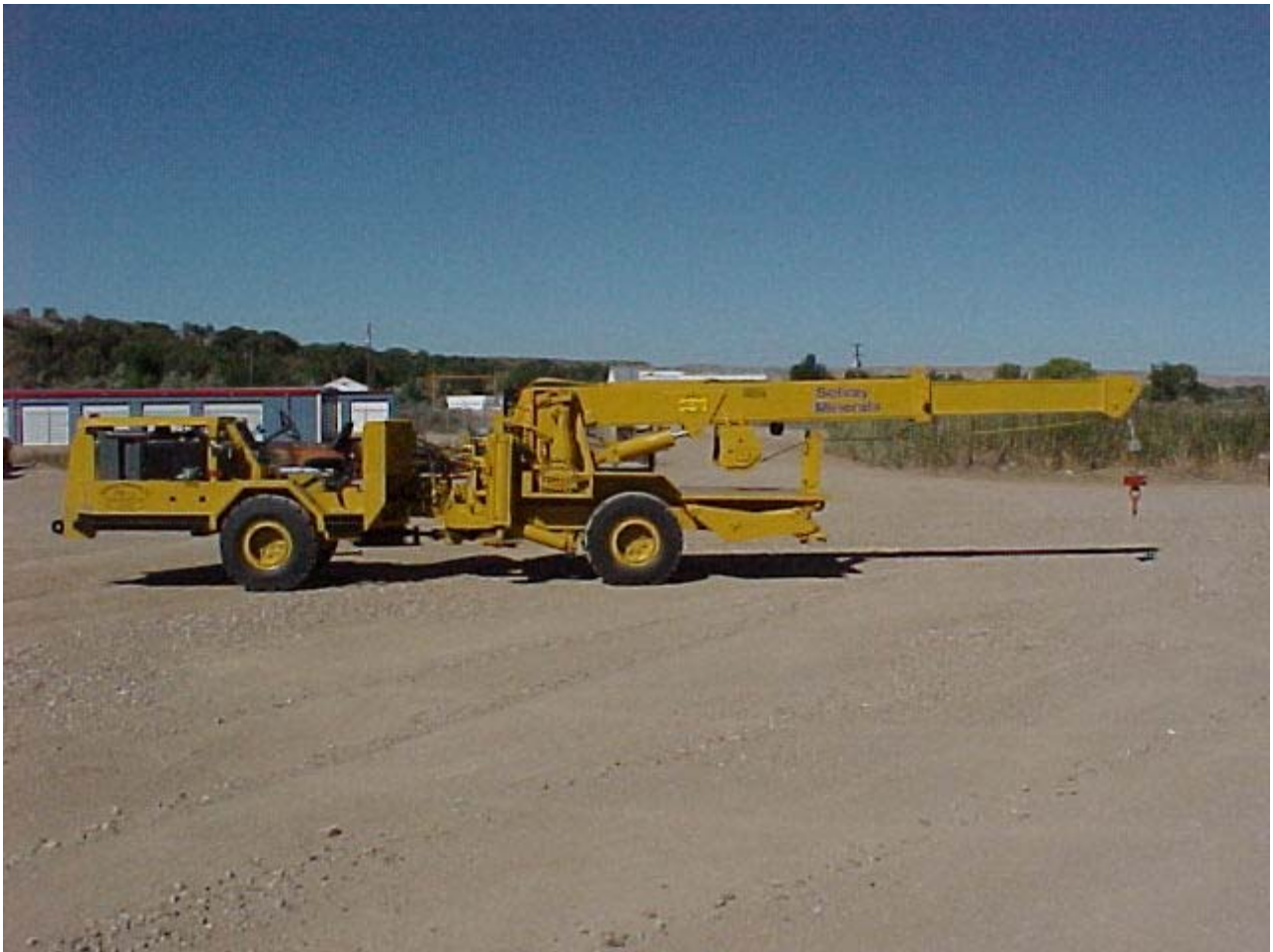
CRANE MODULE DESIGNED & BUILT BY UINTAH MACHINE
