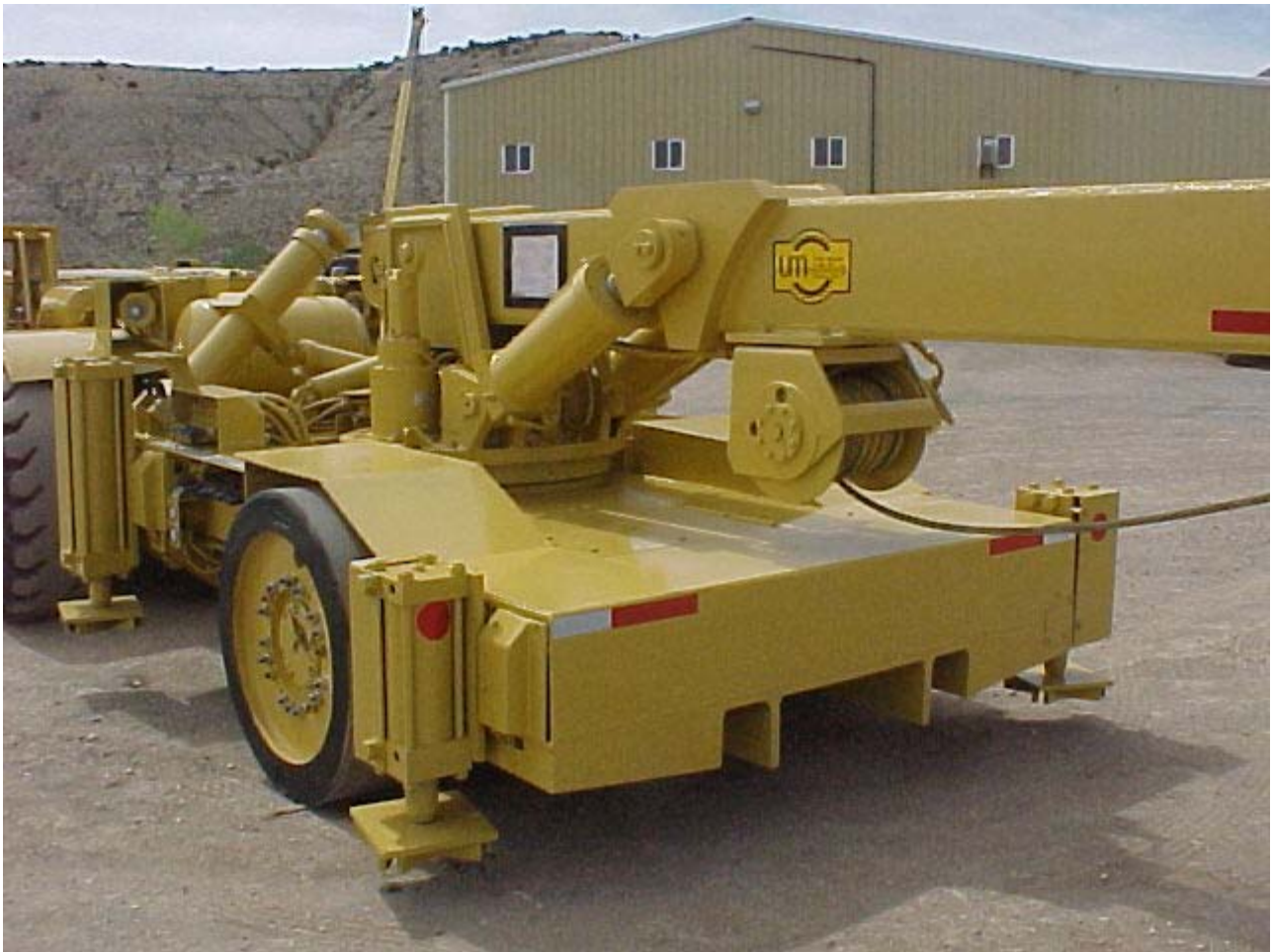
UNDERGROUND CRANE DESIGNED AND BUILT BY UINTAH MACHINE
