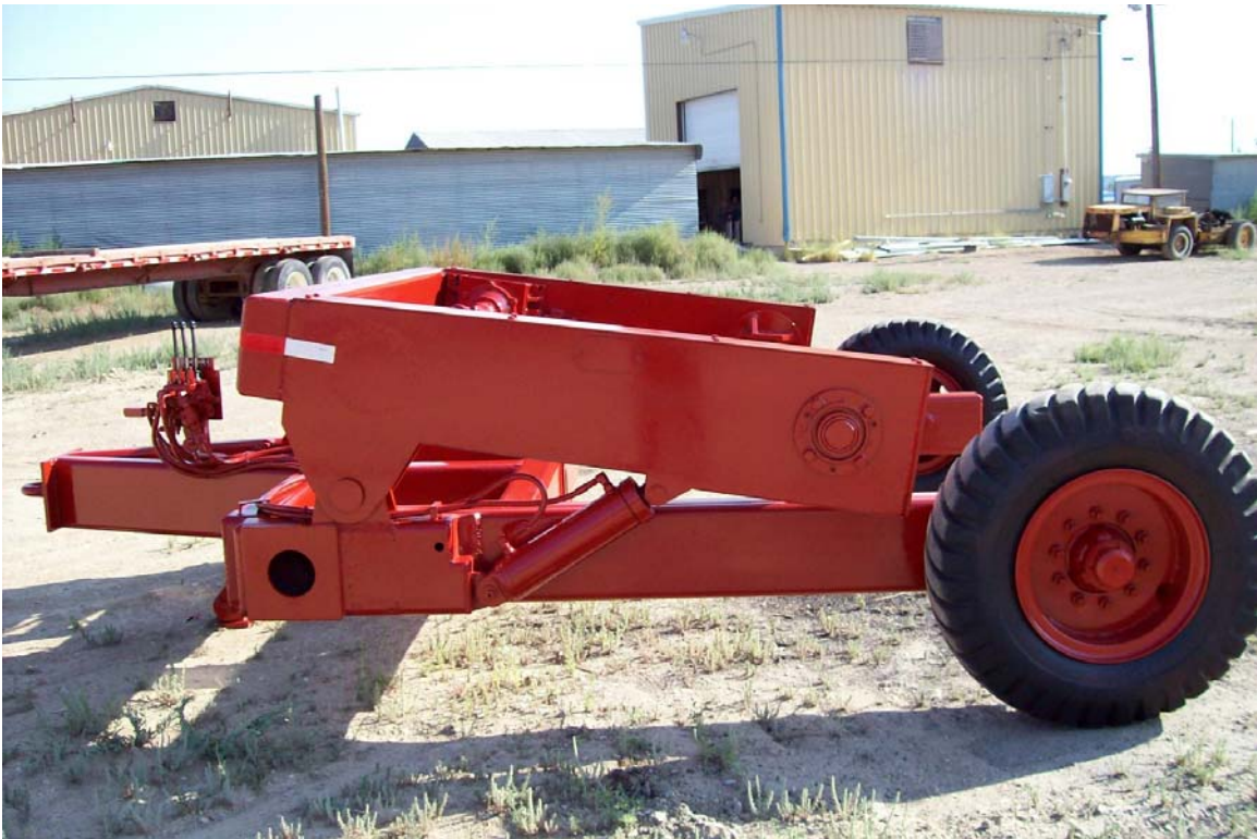
Trailer-type belt winder built on WO # 23906
