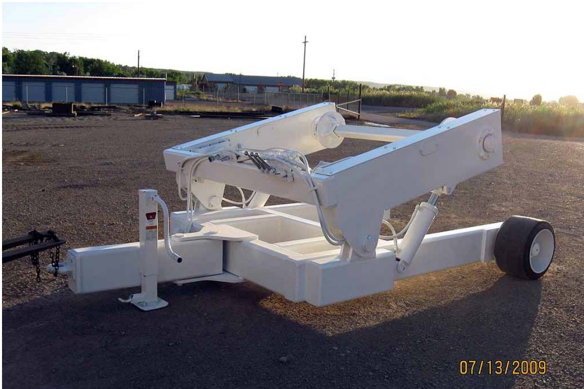
Trailer type belt winder built on WO # 25618
